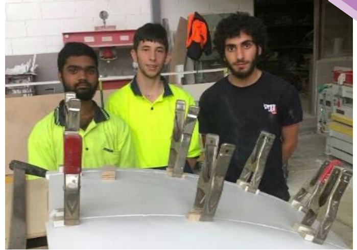
Students Zafir, Peter and Omar of Cecil Hills High showing how they glue and set shaped pieces of Corian for a new Espresso Bar in Darling Harbour
