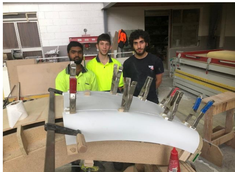
Students Zafir, Peter and Omar of Cecil Hills High showing how they glue and set shaped pieces of Corian for a new Espresso Bar in Darling Harbour
